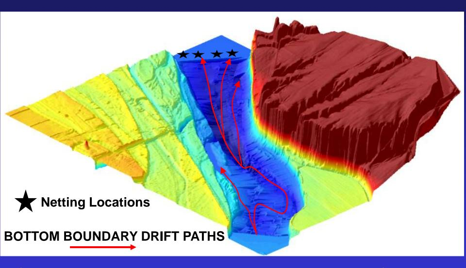
Channel Bathymetry with Floodplain Topography from LiDAR, Informs Calculation of Larval Drift Speed and Pathways
